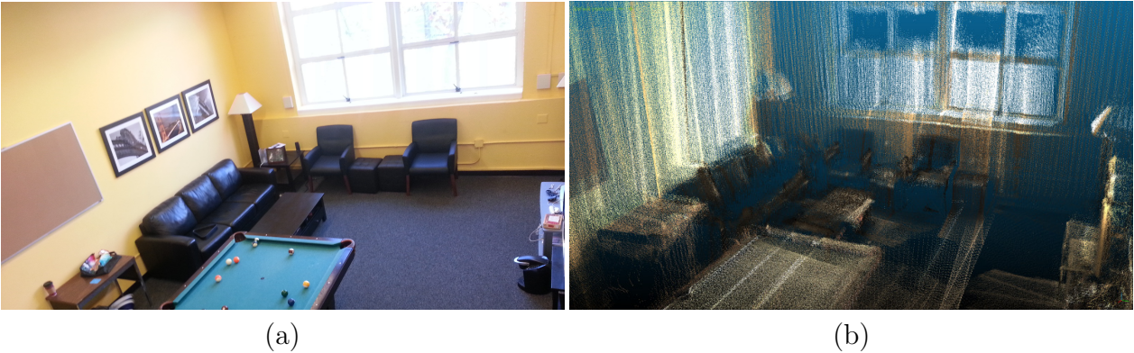
Figure 2.6: A point cloud colored by nearby camera imagery.
