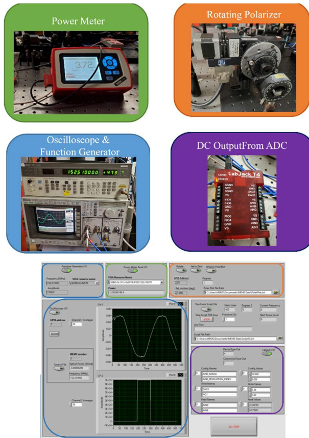
Figure 20: LabVIEW control panel showing controls for the function generator an oscilloscope (BLUE, BOTTOM LEFT), power meter (GREEN, TOP LEFT), rotating polarizer (ORANGE, TOP RIGHT), and analog to digital converter (PURPLE, BOTTOM LEFT).[8]
