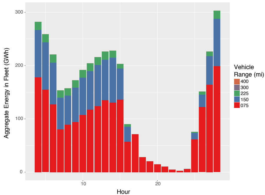
FIGURE 7 Aggregate energy stored in national fleet batteries by vehicle range by hour of day.
