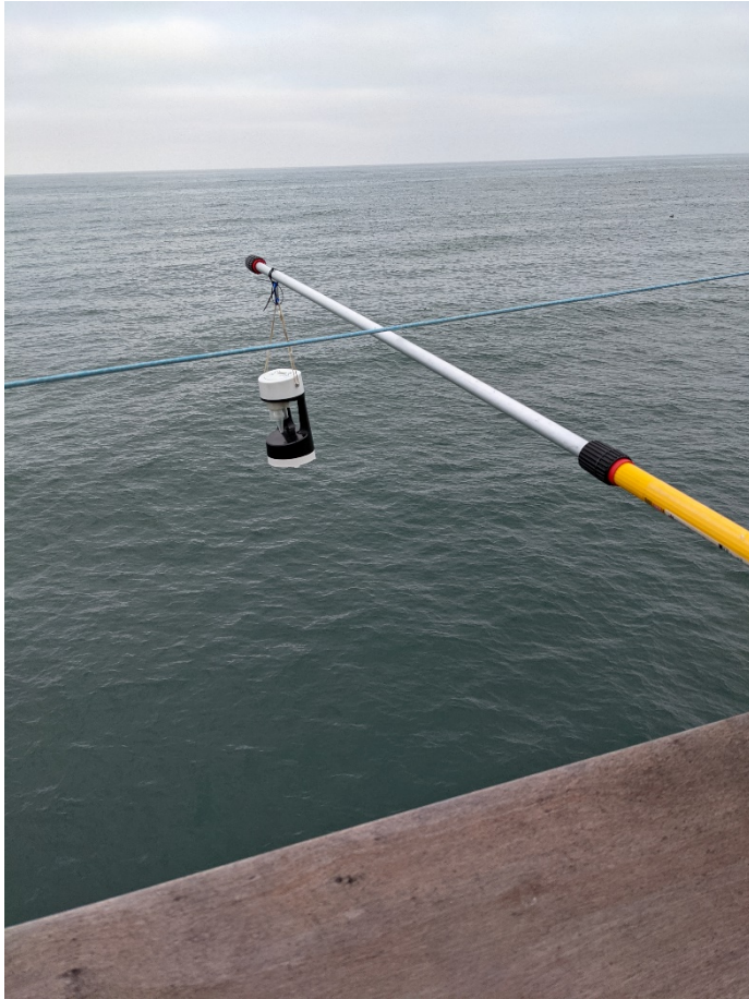
Figure 1: Deployment of Bertin Coriolis Compact (CC). The CC was Deployed from the North end of the Scripps Pier. Daily Samples were collected during a six and a half hour continuous sampling period.
