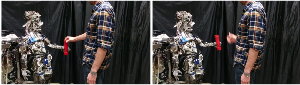
Figure 5.19: Response of the VDNN controller to grasping the decoy object. The left image shows the position of the arm at the start of the grasp, which is the desired location. The image on the right shows the object at its farthest displacement from the desired trajectory.
