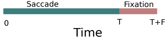
Figure 3.2: Finite horizon time segments. The two segments of the finite horizon used for control. First, from time 0 to time T , there is no penalty for the distance from the eye to the target. Second, during fixation (from time T to time T + F ), the penalty on the eye position is enforced. The penalty on the magnitude of the action U is enforced for the entire horizon.
