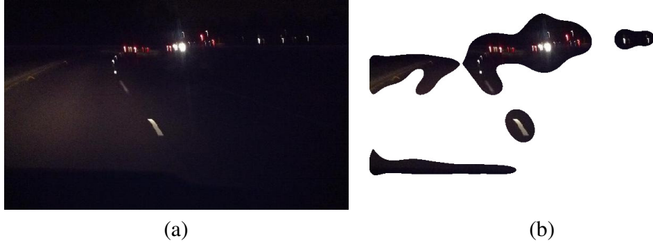
Figure 2.1: (a) A typical night driving scene in San Diego. (b) Image regions expected to provide the most motion information.
