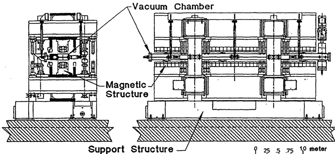
Fig. 1 W16.0 Wiggler end sectional and elevation views
