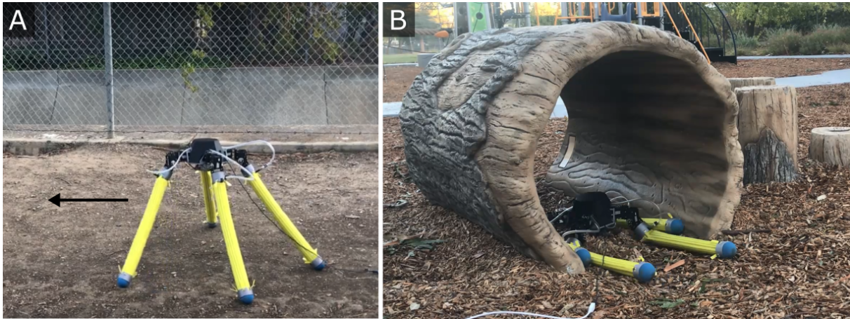
Figure 5.1. Photos of an eight-degree-of-freedom quadrupedal robotic platform with jamming-reinforced inflatable beams limbs. Layer jamming sections run longitudinally along each leg to improve the stiffness of the high-aspect ratio beams when they are pressurized without compromising the desired low-stiffness state of the deflated beams, allowing for navigation of constrained environments. (A) Legs are pressurized to provide improved locomotion speeds and better obstacle traversal capabilities. (B) Depressurizing the limbs allows the robotic system to move through environments that would be inaccessible to a larger rigid robot.
