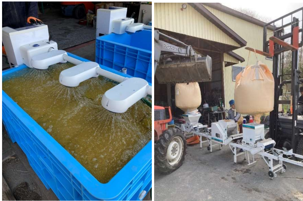
Images: Rice sacks in a germinating machine (left). The seed nursery machine in action (right).
