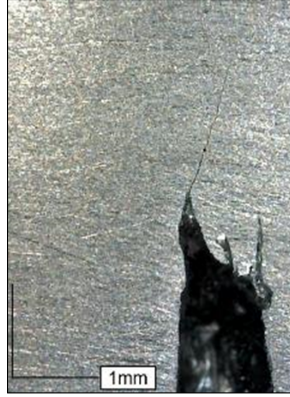
Figure 6: Crack nucleation from the notch at the rivet hole.
