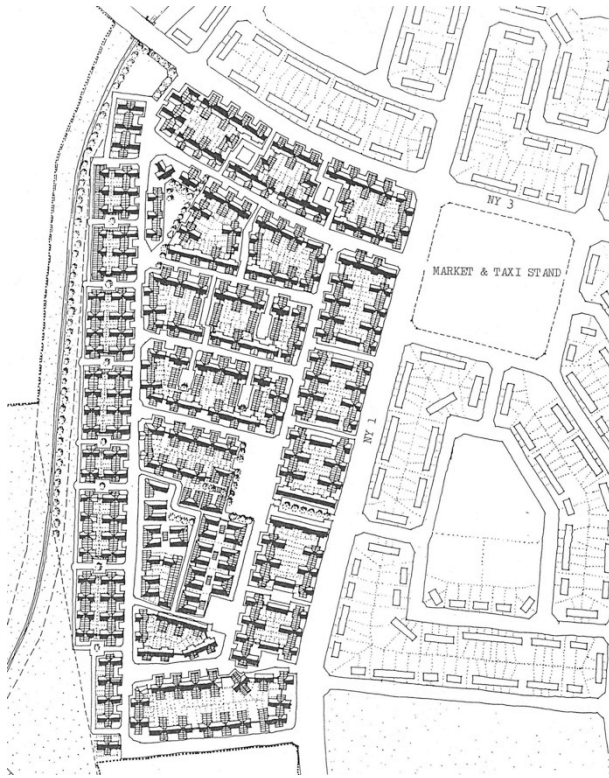
Figure 2.11 Gugulethu Upgrade Proposal. Included in the 1987 Report on the Western Cape Migrant Labour Hostel Upgrade Programme, the proposed upgrades to Gugulethu suggested filling the space between the existing buildings (shaded) with new buildings to create more housing and to create pedestrian-scaled outdoor spaces that would foster social interaction. From Western Cape Hostel Dwellers' Association 1987.
