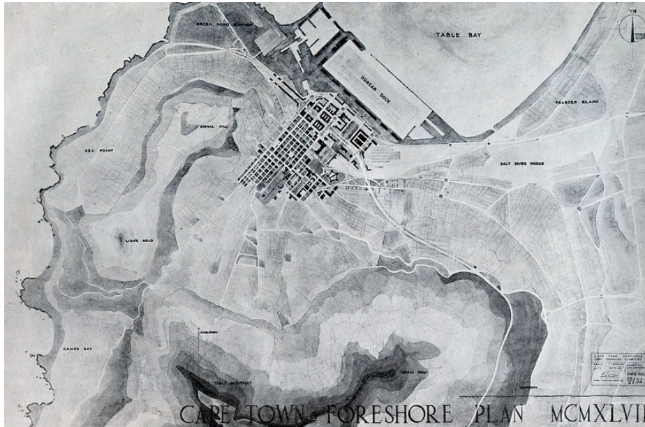
Figure 1. The Foreshore Plan, drawn by J.H.C. Hofmeyr, 1947. The Foreshore and Duncan Docks filled in Cape Town's natural harbor to create a modernized industrial port and new central business district area. From http://farm5.static.flickr.com/4030/4500664364_310a0f8418_b.jpg .
