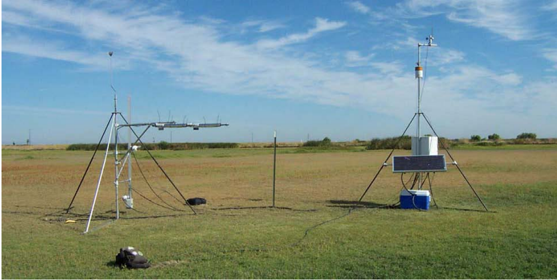
Figure 5. Bowen weather station showing the solar panel, 6V batteries (inside the cooler below to prevent contact with moisture), cable box with datalogger, rain gauge, and anemometer. Two net radiometers (left side of photo) are held at approx. 1.5 m over the surface. The air exchangers (right side of photo) face the prevailing winds and are spaced 1 m apart, with the lower exchanger positioned approximately 25 cm above the surface.
