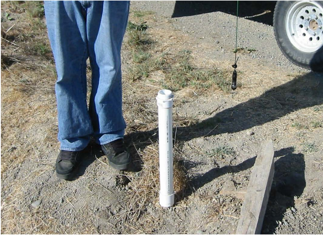
Figure 6. Deployment of pressure sensors in shallow groundwater monitoring wells to measure changes in water table depth and to estimate pond seepage losses during fall flood-up.
