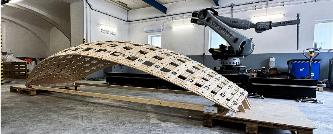
Figure 10: Completed bending-active formwork with 9 longitudinal and 22 transverse timber strips.
