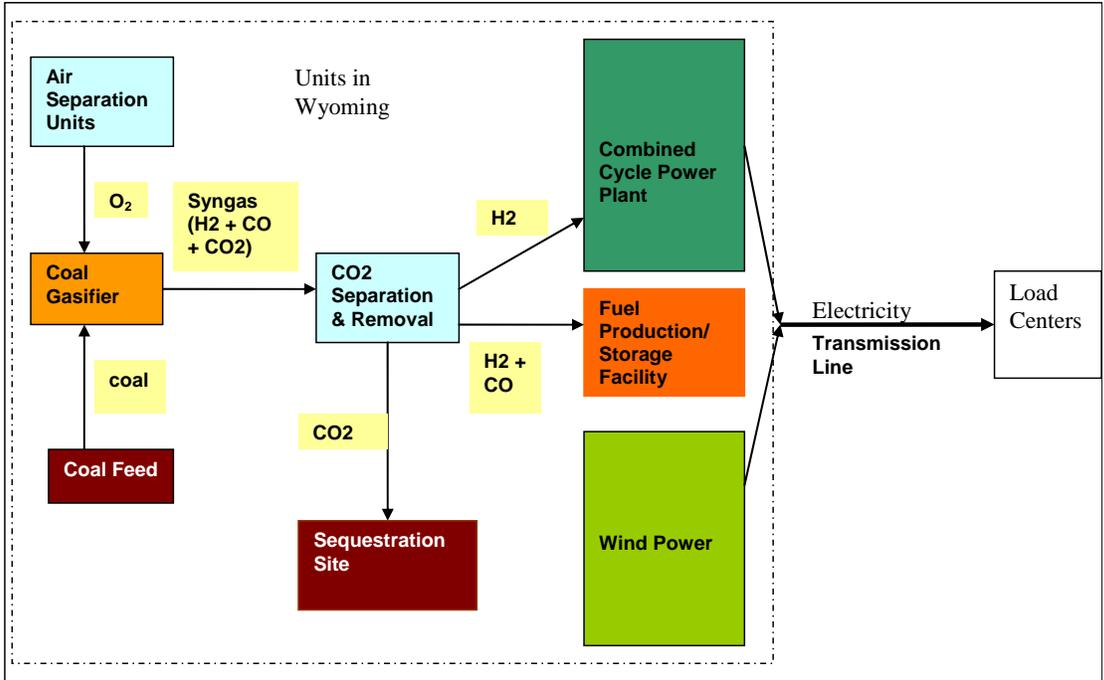
**Figure ES-1. Advanced Coal Wind Hybrid: Basic Configuration**
