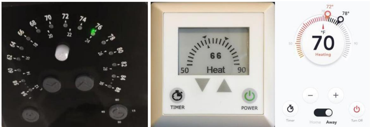
Figure 1. Current temperature (pictured left to right: first hardware; second hardware; mobile application).
