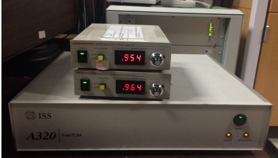
Fig. 5.7: Fast FLIM system (ISS) with a digital frequency domain (DFD) approach and equipped with standard light detectors
