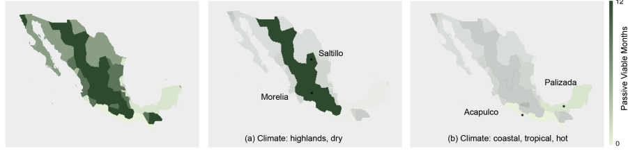
Fig. 4. Passive-viable months for top-performing construction for each location. (a) high-performing construction in Saltillo and Morelia (façade: HP masonry unit, adobe; roof: concrete (insulated)), (b) high-performing construction in Acapulco and Palizada (façade: brick wall; roof: corrugated metal (insulated)).
