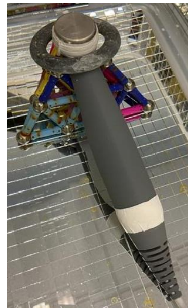
Fig. 4.2 SAT setup with a high-frequency probe sonicator for biofilm treatment. The probe was immersed in a water bath, and the temperature was monitored during the experiments with a
