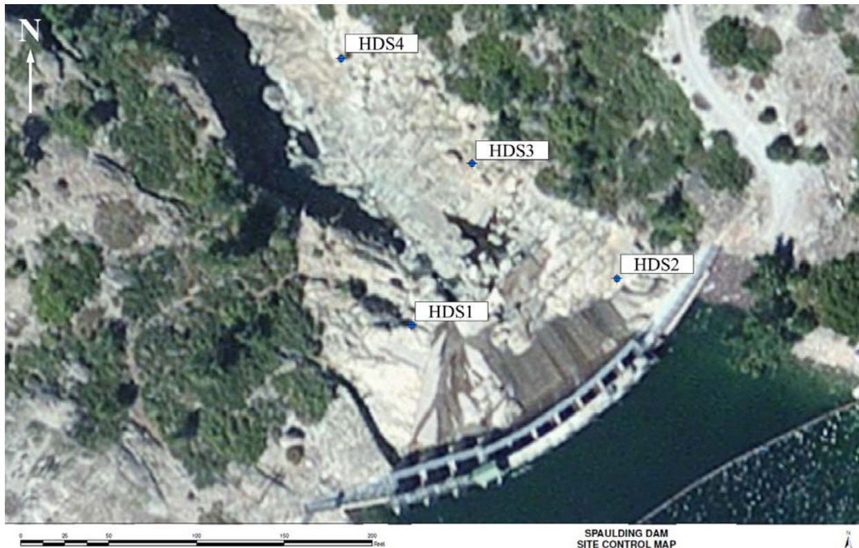
Figure 3-21. Spaulding Dam No. 2 survey control points (provided by AMEC).
