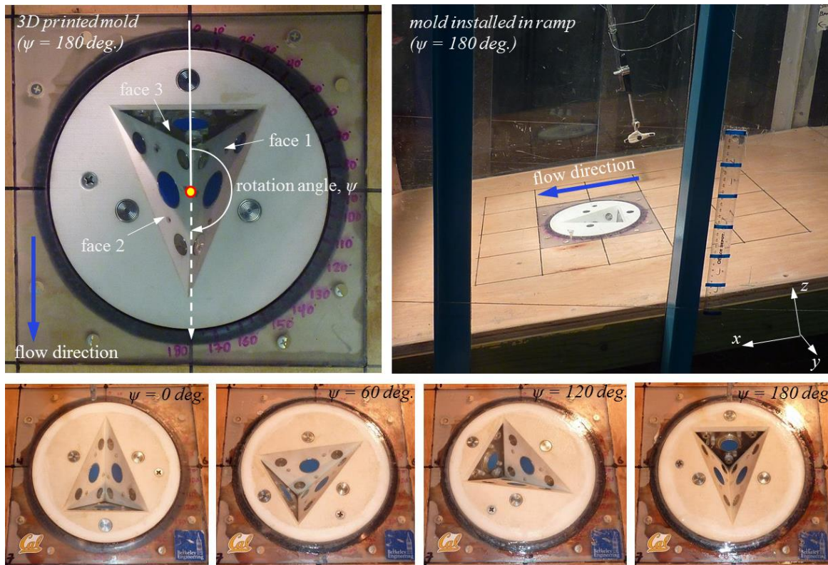
Figure 4-4. 3D printed block mold with acrylic face (top left), installed in ramp (top right) and rotated at angles of 0, 60, 120, and 180 deg. (bottom left to right).
