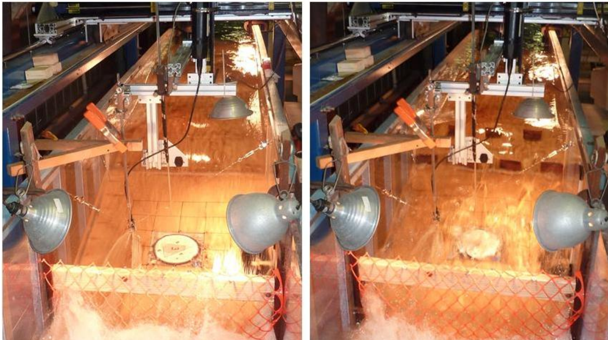
Figure 4-11. Low ( T_u = 2.2\% , left) and high ( T_u = 7.4\% , right) turbulence conditions for Q_9 looking upstream from downstream end of steep ramp section.
