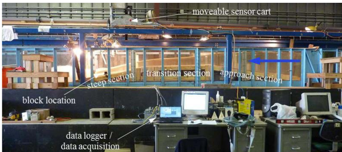
Figure 4-2. Ramp constructed inside flume at RFS.
