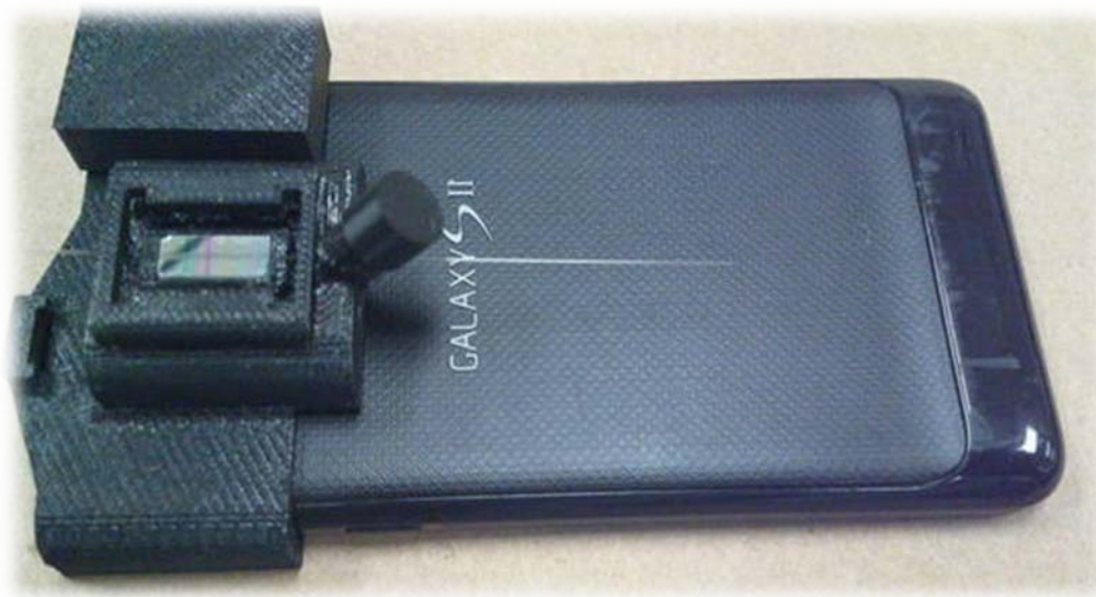
Figure A-9 | The entire optofluidic imaging multicolor cytometer on a cellphone.
