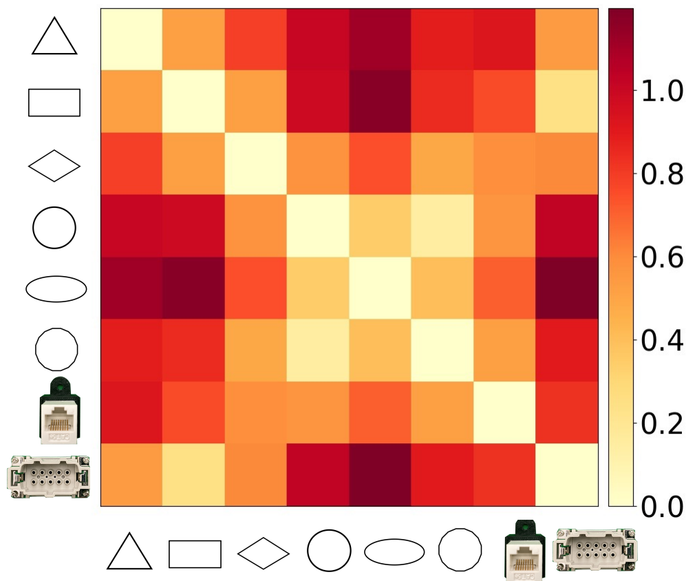
Figure 5.6: The similarity distances between all insertion tasks. Given a new task, we use the obtained similarity distances to select similar tasks from the existing task library and transfer the task knowledge, i.e., primitive parameters, to the new task.
