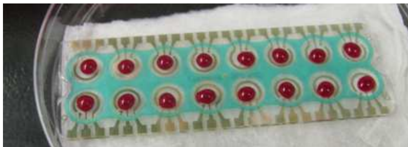
Figure 18. Photograph of the 16-array Genefluidics array electrode with a plastic well (in green) separating the individual electrodes. Whole blood samples are being incubated on the surface of the electrode chip, where upon completion of incubation wash off blood will be performed with distilled water. The remaining portions of the assay after this sample incubation step are the incubation of a detector antibody in casein/PBS, the washoff of unbound detector antibody, and pipetting of tetramethylbenzidine/ H_2O_2
