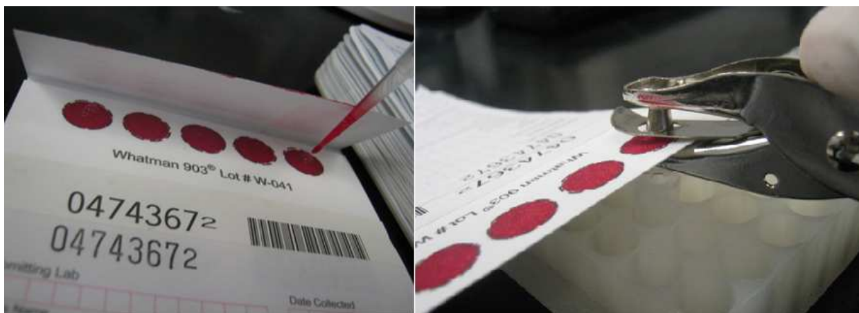
Figure 40 Dried blood spot reconstitute. Left figure illustrates the pipetting of 60 \mu\text{L} of whole human blood on the surface of the proteins saver card. Right figure illustrates the hole punching of the dried blood spots on the filter paper into a microcentrifuge tube before shaking at room temperature.
