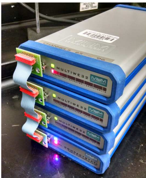
Figure 1 Potentiostat units interfaced together. The electrochemical interface for this experimental setup utilizes three multiplexing modules on top of the CompactStat electrochemical potentiostat. These are interfaced together by a ribbon cable, and the multiplexing modules are connected to electrodes via a 37-pin D connector system located on the rear of the modules.
