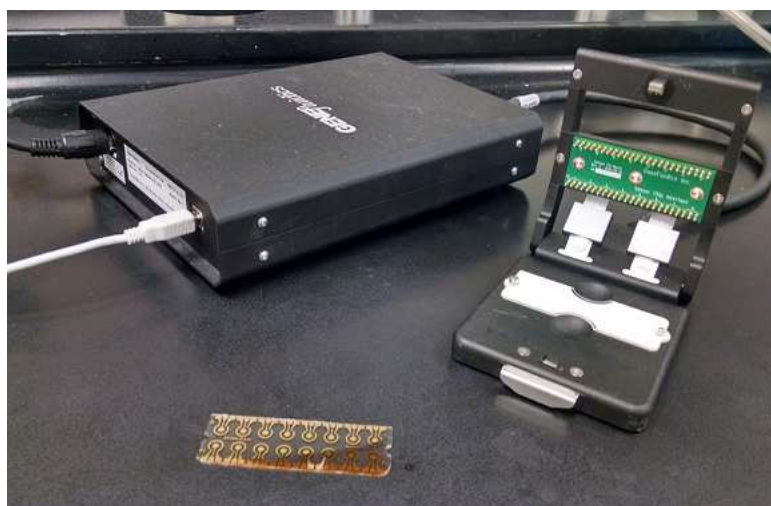
Figure 17. The Genefluidics 16-array electrochemical platform that was used in the initial phases of experimentation. This is a well-validated electrochemical system that has been widely applied to a variety of detection contexts, and serves as an initial first platform for evaluation of the electrochemical assay method prior to tests for adapting the electrochemical method to a more high-throughput context.
