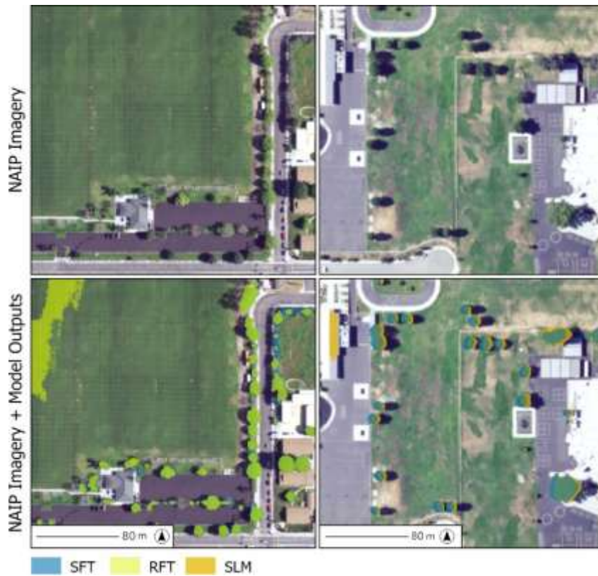
Figure 2.3 Example model outputs for canopy segmentation on NAIP imagery. The top panel shows the NAIP image tile, with a corresponding bottom panel with transparent model outputs overlaid together. Left: The statewide fine-tuned model (blue) overlaid under the regionally fine-tuned model (yellow). RFT has more artifacts, and under predicts canopy, but is sometimes more precise than SFT. Right: SFT (blue) overlaid on top of the output from the statewide LiDAR model (SLM, orange). SLM produces artifacts on rooftops and tends to overpredict canopy in shadows and beyond the extent of the tree compared to SFT.
