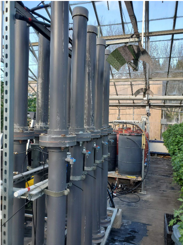
Figure A-5. The slow sand filtration system on the left, water storage in the background, and chrysanthemum beds on the right.
