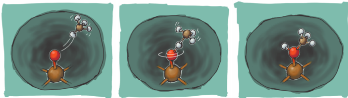
Scheme 1: A schematic representation of the rebound mechanism for the conversion of methane to methanol over Fe-oxo sites. After initial adsorption of the molecule (left), one hydrogen is abstracted before an intermediate (middle) is formed. Methanol (right) is formed after the so called rebound step, where the OH-group rotates around. O atoms are displayed in red, Fe atoms in gold, H atoms in white and C atoms in brown.
