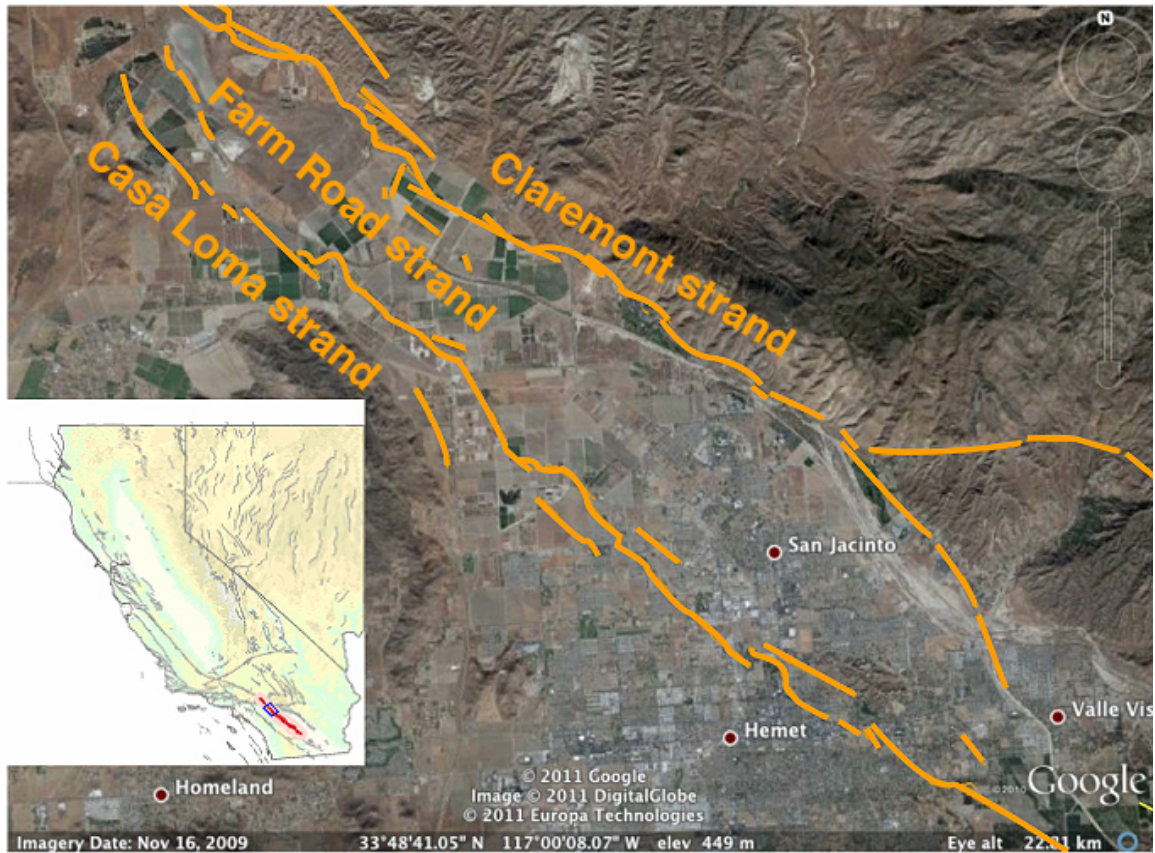
Figure 2.1. The Claremont-Casa Loma stepover of the northern San Jacinto Fault, southern California: a real-world example of a stepover with an intermediate fault strand between the primary segments. The rightmost strand is the Claremont, while the leftmost is the Casa Loma. The small fault between the two main strands, in the upper left of the image, is the Farm Road strand (USGS, 2010).
