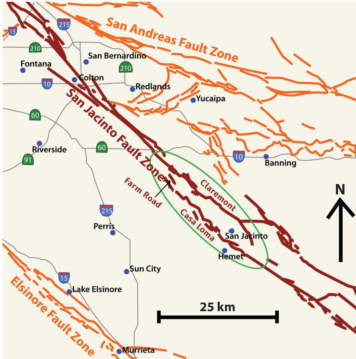
Figure 3.2. Close up of the northern San Jacinto Fault Zone. The Claremont-Casa Loma stepover is circled in green. The Claremont strand is the more northeasterly of the two; the Casa Loma is to the southwest. The small fault within the northern end of the stepover is the Farm Road strand.
