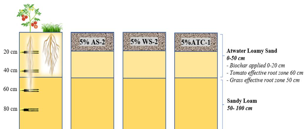
Figure 3-1 Conceptual diagram of HYDRUS 1-D simulation domain demonstrating control and biochar amendment scenarios for two cropping systems.
