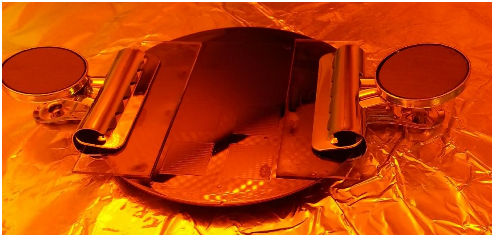
Figure 5.11: Exposed Bonding Process. Glass slides are clamped onto wafer, and an additional weight is placed on top afterwards to add pressure to bond the layers of SU-8 together.
