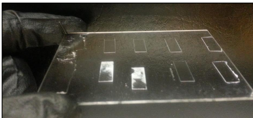
Figure 5.1: UV Filter Characterization Test Slide. For the ten positions, there are two control positions along with eight test sites. The two cloudy samples represent the lowest energy levels that were not fully exposed, while the other six sites are fully exposed. The two test samples on the far left were not processed correctly and were unmeasurable.
