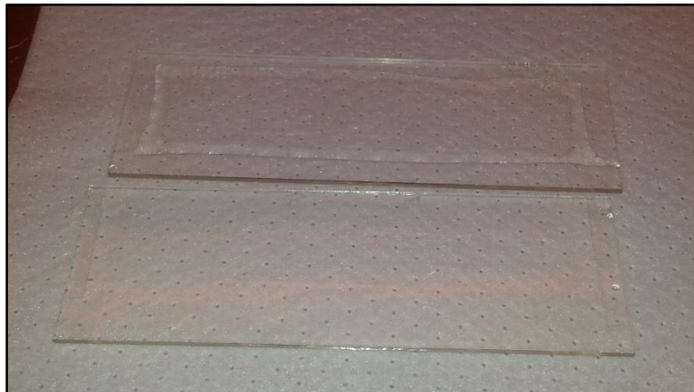
Figure 5.2: SU-8 3050 on SU-8 3005. The top slide shows an uneven layer of SU-8 3050 on top of 10 \mu m layer of SU-8 3005. The bottom slide is a single 10 \mu m layer of SU-8 3005.
