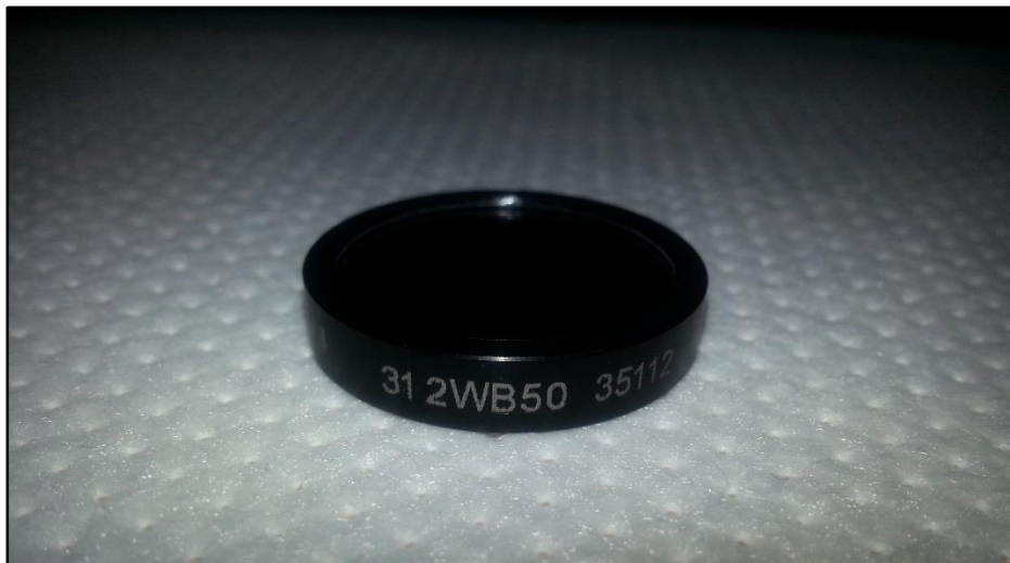
Figure 3.6: 312 nm UV Filter. The UV Filter is a small circular disc that is placed on top of our pattern, limiting the wavelengths of light that will expose the pattern on the SU-8 layer.
