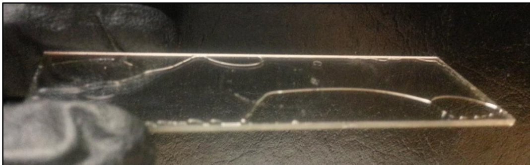
Figure 5.7: SU-8 3005 on SU-8 3005. After complete processing of the first 10 \mu\text{m} layer of SU-8 3005, the second layer of SU-8 3005 did not evenly disperse during spin coating.
