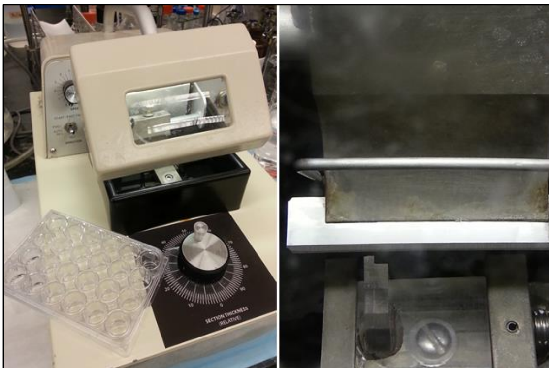
Figure 6.8: Vibratome Setup. (Left) The vibratome features dials to control the speed of the blade and section thickness, and a multi-well plate is used to store sample slices. (Right) Through the 2x magnification lens, we can see the blade as it approaches the sample, which has been glued to a plastic substrate to maintain proper positioning. (Facility: Glabe Lab at UCI.)
