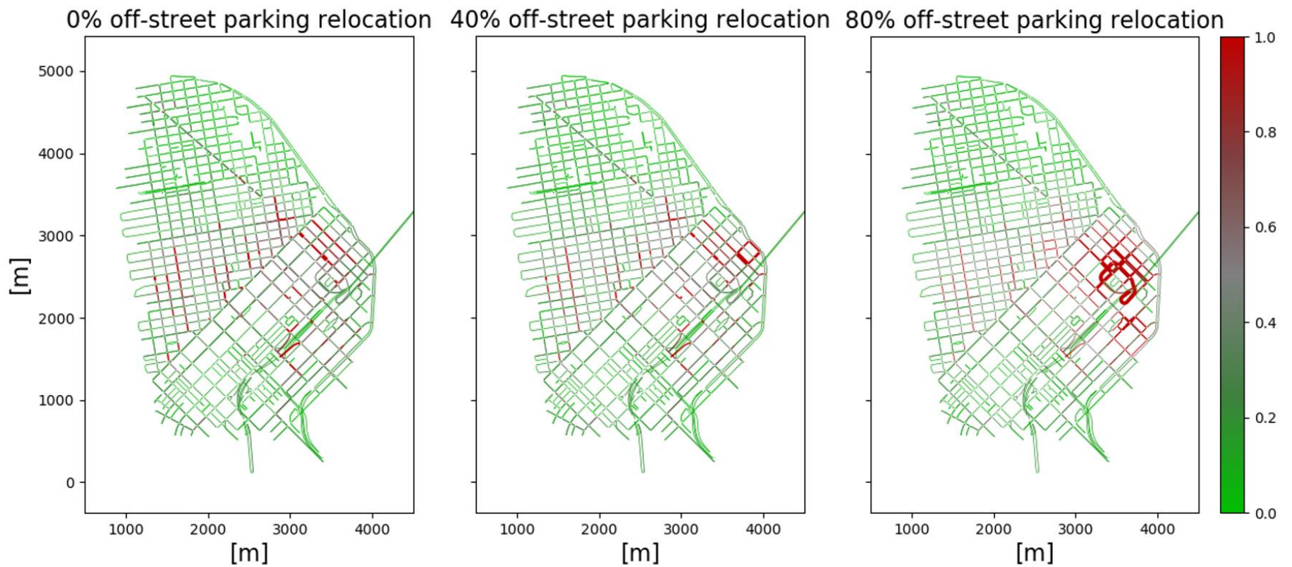
Figure 7. Average daily roadway link-level occupancy results for scenario set 3 (conversion of 0%, 40%, and 80% of on-street parking spaces to drop-off/pick-up spaces).
