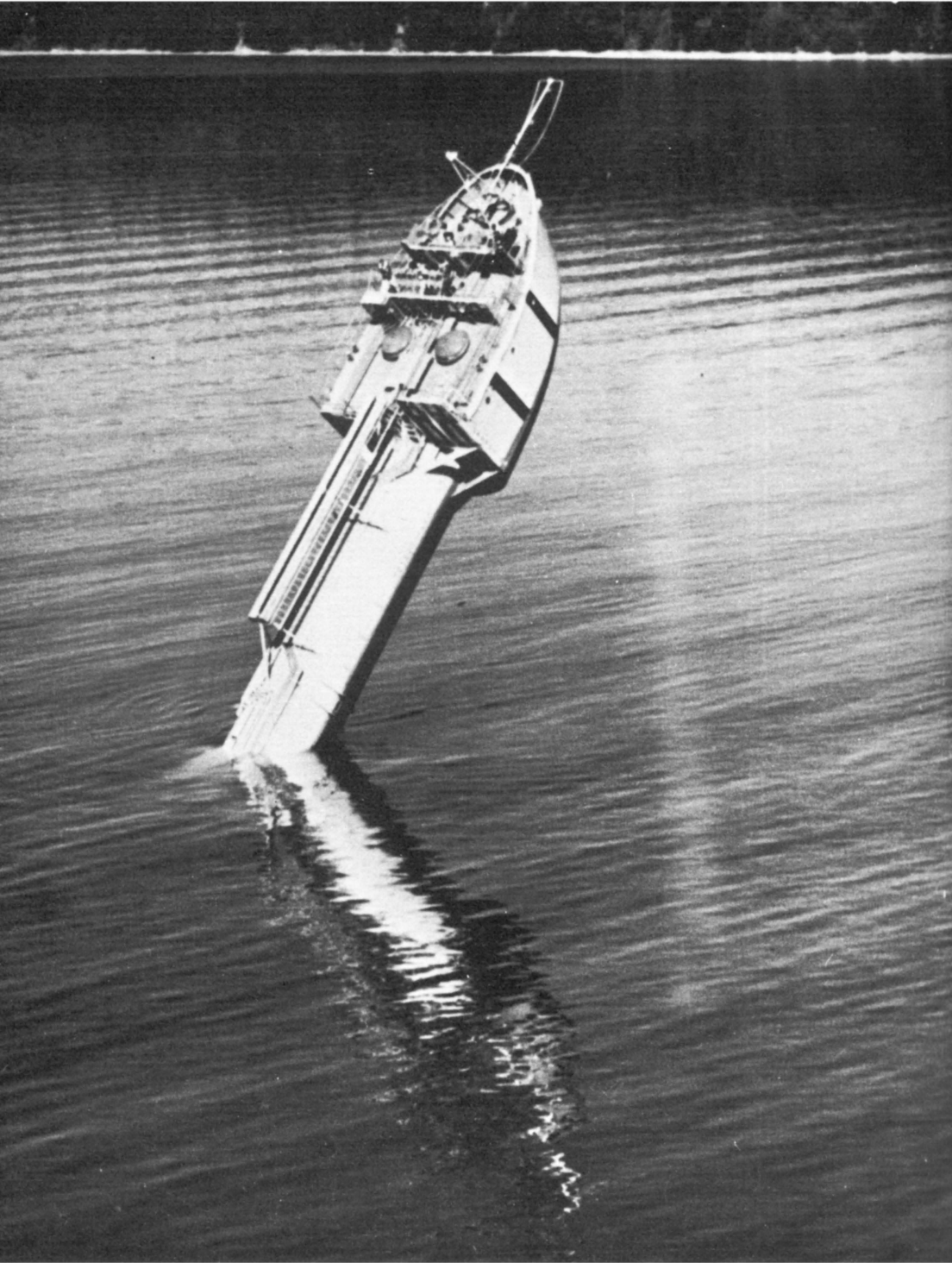
FLIP, Floating Instrument Platform is returning to the horizontal. When in the vertical position she displays only 55 feet of her total 355-foot length. FLIP has no motive power of her own, is towed to station.
