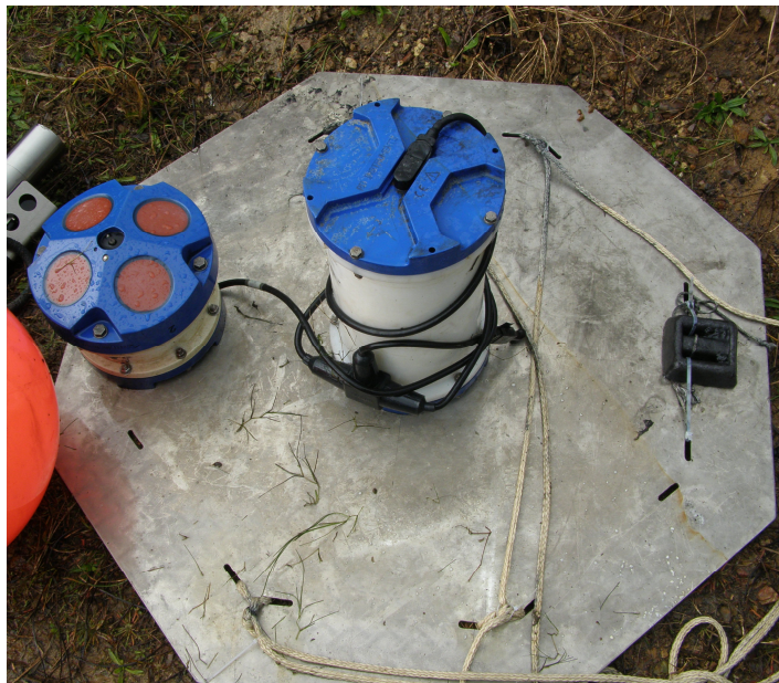
Fig. 2-8. Approximate deployment configuration for the RDI 1200-kHz ADCP in April 2008, mounted upward-looking on a flat plate. The battery pack orientation differed from that shown here.
