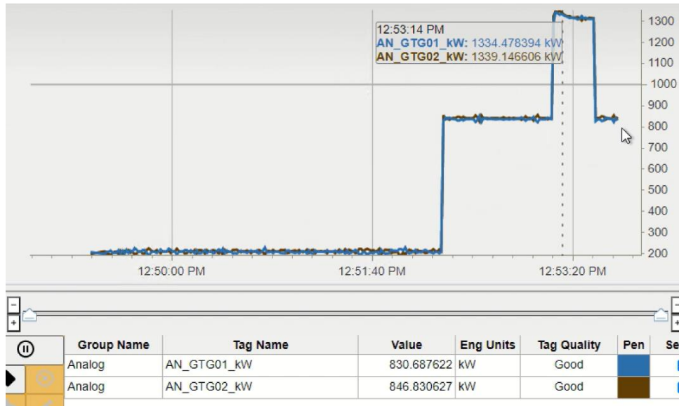
Figure 41 GTG 1 and 2 ramp-up to provide black start charging for BESS
