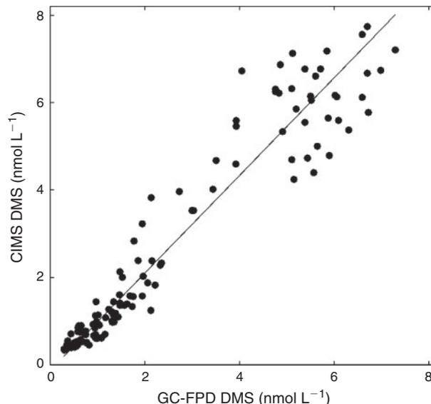
**Fig. 4.** Model II regression for equilibrator and atmospheric pressure chemical ionisation mass spectrometer (Eq-APCIMS) against gas chromatography with flame photometric detection (GC-FPD) dimethylsulfide (DMS) concentrations in 125 samples;  $y = 1.12 (\pm 0.03)x - 0.13 (\pm 0.09)$ ;  $R^2 = 0.92$ ;  $P < 0.0001$ .
