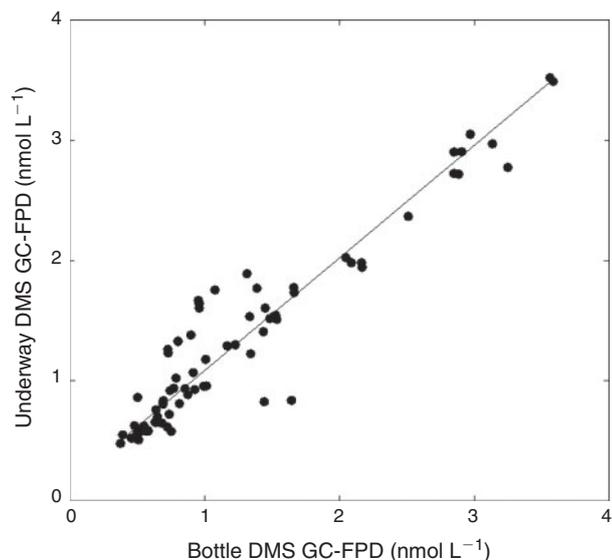
**Fig. 5.** Model II regression for underway dimethylsulfide (DMS) sampling against co-located overboard bottle sampling using gas chromatography with flame photometric detection (GC-FPD) for the analysis of all 75 samples;  $y = 0.94 (\pm 0.024)x + 0.15 (\pm 0.036)$ ;  $R^2 = 0.91$ ;  $P < 0.0001$ .
