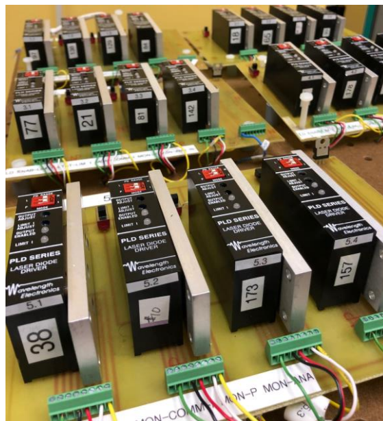
Figure 20: Picture of the laser diode drivers. The drivers are grouped into five groups of four drivers based on their corresponding operating wavelength.
