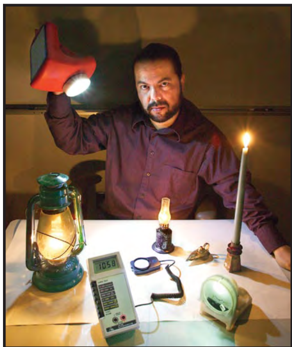
Figure 1. Evan Mills holds a prototype white light-emitting diode (WLED) made by a company called Ignite Innovations. This lamp, which grew out of a Stanford-led effort involving several Silicon Valley companies, Berkeley Lab, and others, features a one watt WLED, solar panel and rechargeable AA batteries. (Photo by Roy Kalischmidt)
