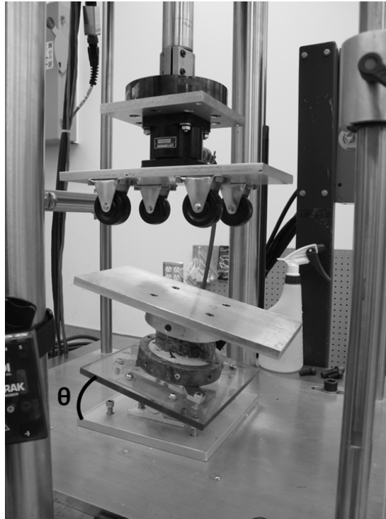
Figure 3.1: Image of custom jig to impose postures implicated in disc herniation on motion segments. Linear actuator lowers and each of four caster rollers make contact with plate sitting atop motion segment to impose compression and a flexion angle \theta .
