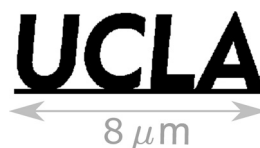
FIG. 4. The geometry of the target used for mass contrast imaging is shown in black, and a scale bar is shown in gray. In order to calculate the effect on the electron beam (angle scattering and energy loss), the sample is assumed to be a 20 \mu\text{m} thick Cu.
