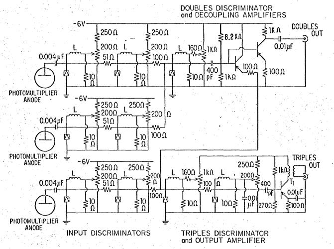
All Tunnel Diodes are TD 119 (RCA). All Transistors are Philo 2N769. Trim "L" for desired pulse length 1uH or less. To has 10-turn primary, 5-turn secondary, which are Trifilar wound on Ferroxcube 102 core.
