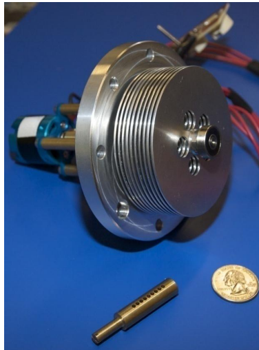
Figure 2.2: Photograph of the Tesla rotor tested with air
