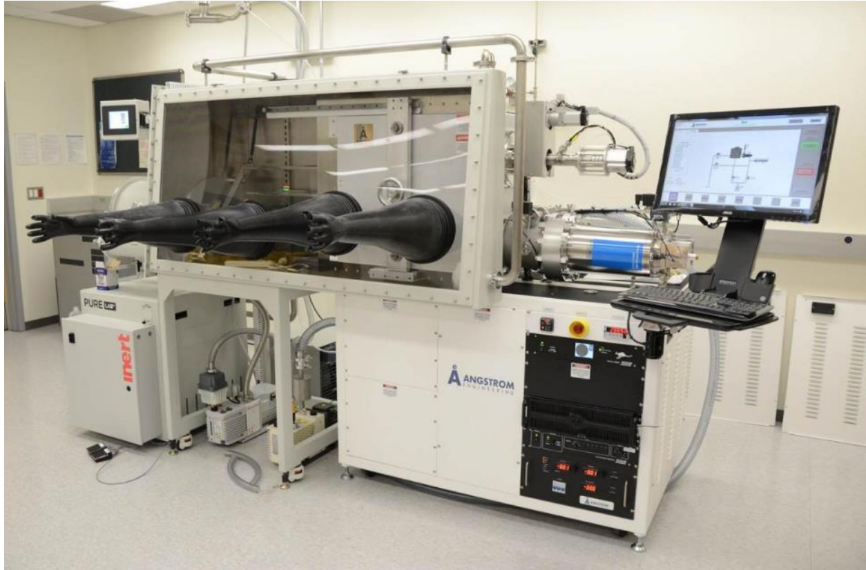
Fig. 2.2 Angstrom Engineering EvoVac Glovebox Evaporator in IMRI.
