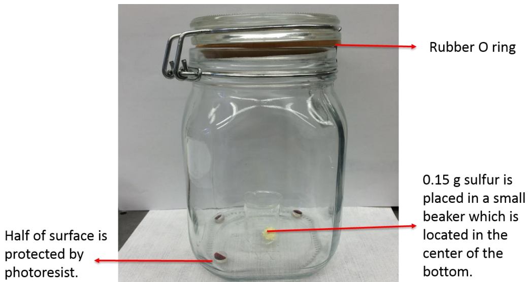
Fig. 3.12 Sulfurization test setup.
