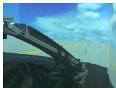
(b) Virtual system using a high fidelity driving simulator
