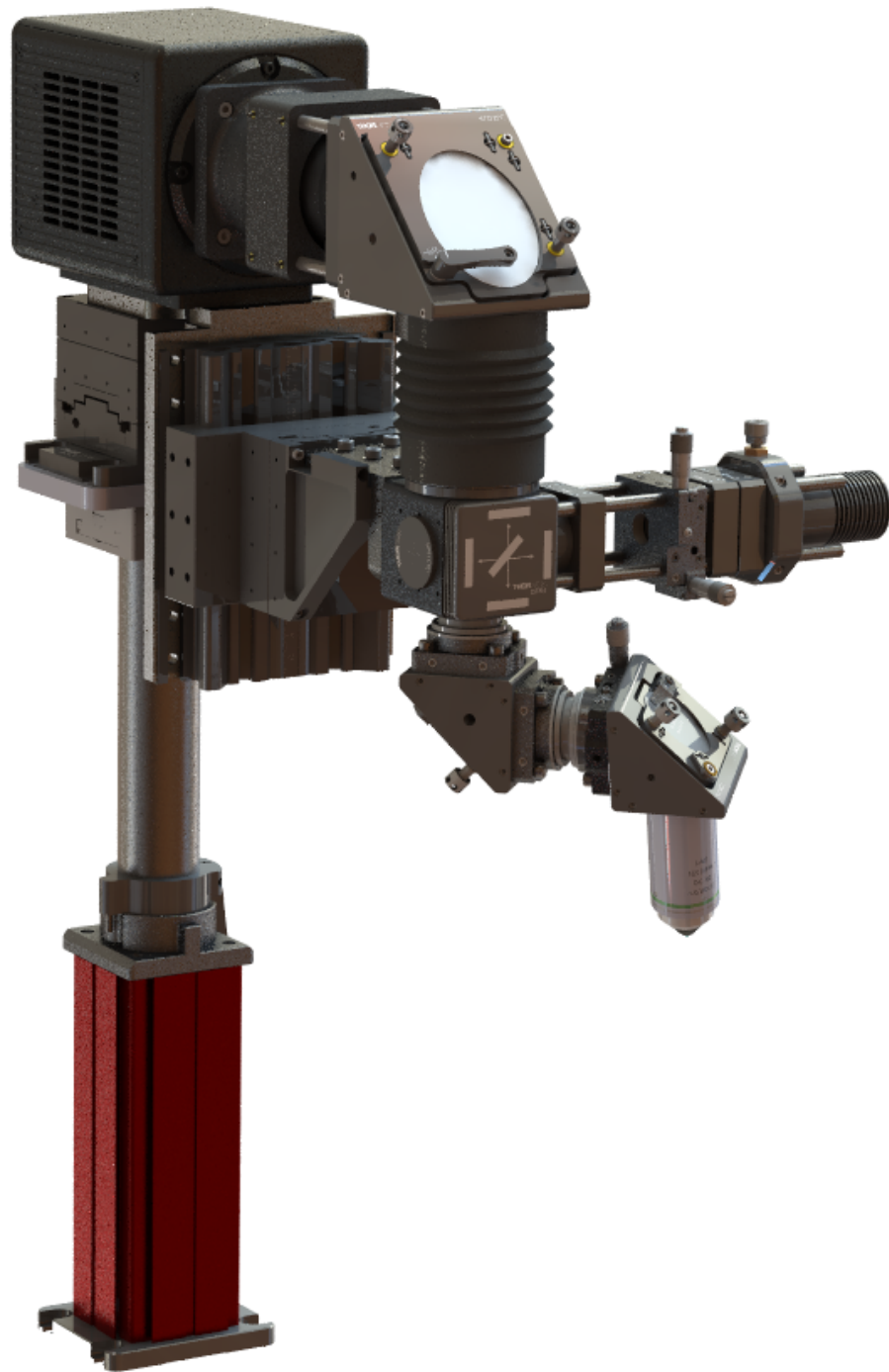
Figure 10.5: Spatially Confined Excitation Voltage Imaging Microscope The system as configured at the University of Toronto. The UCLA version of the system is slightly different with the same fundamental operating principles.
