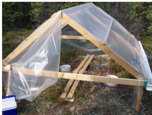
Plate 1 Greenhouse constructed to passively warm boreal forest soils in central Alaska.
