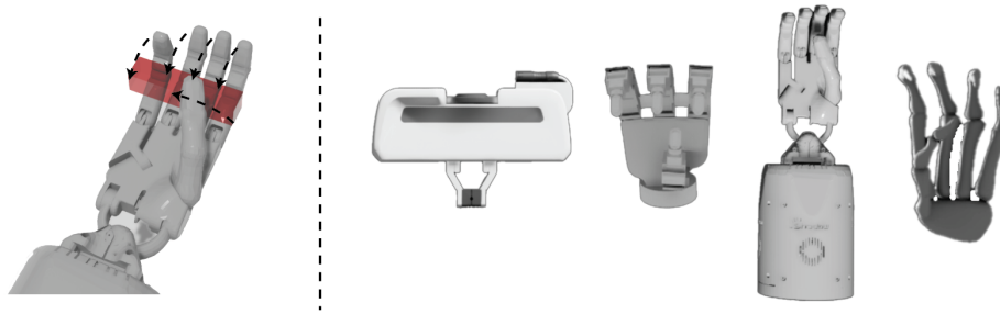
Figure 3.8: Grasp illustration. Left: grasp planner illustration. We regard the handle as a cuboid and the grasp planner searches the joint positions through curling fingers. Right: final grasping states deduced by the grasp planner.
