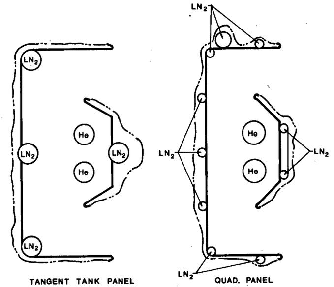
Cryopanel cross sections.
