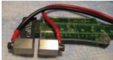
Figure 5.1. Plate electrode used to apply NTIRE across the small intestine. The plate electrodes used for in vivo experiments on the rat intestine are shown. These BTX Caliper Electrodes are produced by Harvard Apparatus (Holliston, MA). When applied across the rat small intestine, the two electrodes are held apart by approximately 1 mm.
