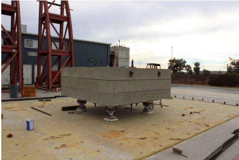
Figure 5.6: Experimental subassembly on shake table
