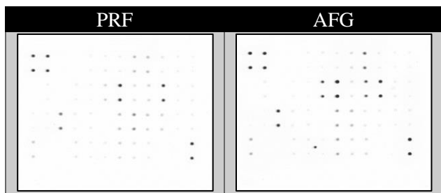
Figure 2. Antibody Array with Chemiluminescence. Example antibody array with chemiluminescence detection. Both PRF and AFG have many growth factors in common but their concentrations differ shown by different level of intensity of each well.
