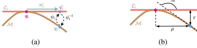
Figure 3.24: (a) A chart C_i operators comprising exponential \psi_i and logarithmic \psi_i^{-1} functions for mapping between the tangent space at q_i and the manifold. (b) The parameters defining the chart validity region.
