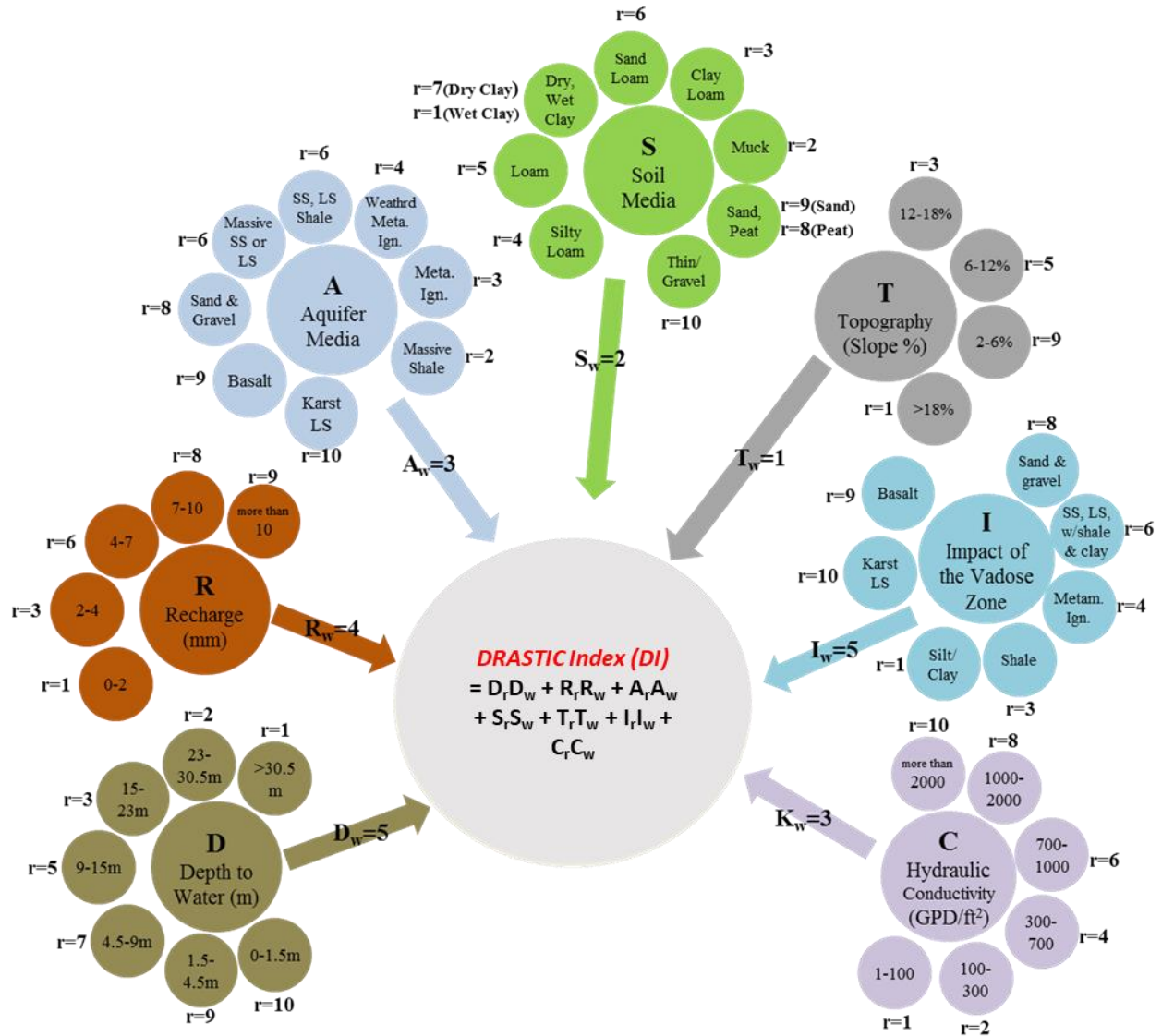
Figure 2: DRASTIC with weights and ranks for model parameters.
