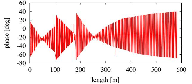
Figure 2: Mean bunch phase at cell centres along the linac
